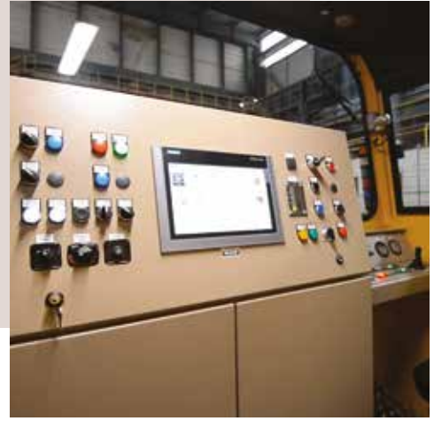
Ergonomic driver desk with joysticks for traction/brake control
